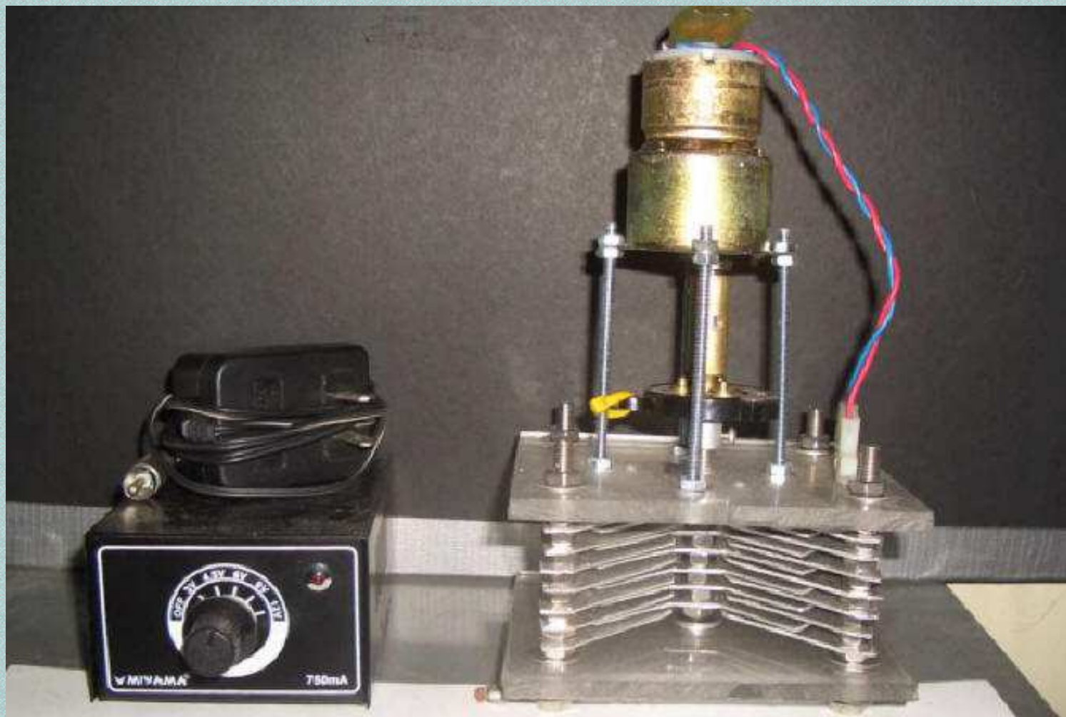
showing the control unit and the motor/gearbox arrangement
